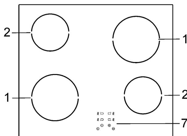
The appliance has 2/4 heating elements of different sizes and power levels. The heating elements are of the Hi-light type, which come on after a few seconds, and the heat is adjusted using the controls on the front panel, from a minimum of 1 to a maximum of 9.
